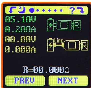
Data Connection Cable Impedance Measurement Interface
