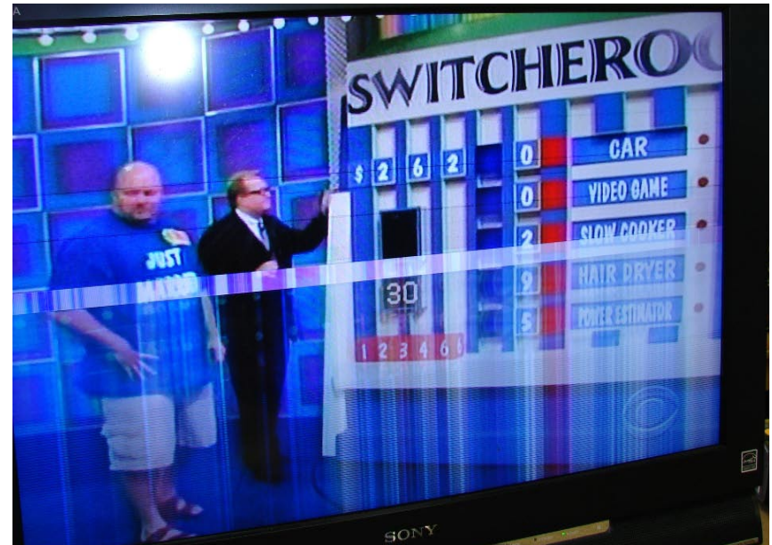
GATE DRIVER FAILURE
