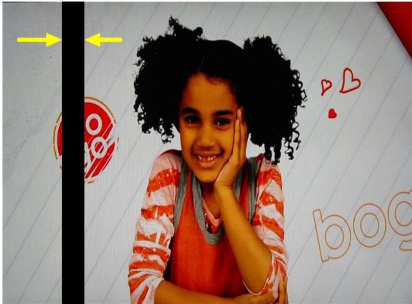
SOURCE DRIVE IC FAILURE
