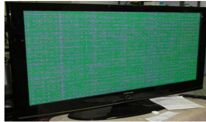
Green lines or a green screen defective main board , LVDS , or T-CON.
