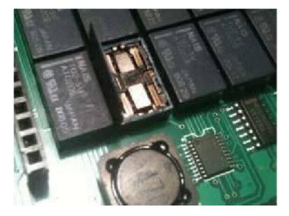
When CDP powered and connected to USB, run SW and connect to any car (no need for a real car!) and then go back to main SW window. measure relay coils and see how many are ON: 3 relays must be ON when in this window! If only 2 are ON BMW E60 and E90 don't work!
