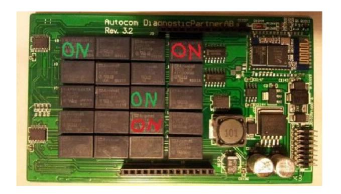
replace relays drivers ic's LV125D > NPX 74LV125D
