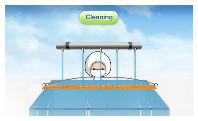
The panels entering the module process are first cleaned with clean water and paper made of organic materials to wash off debris produced during the cell process. The surfaces of the panels are then wiped with a soft brush and air-dried for the next process.
