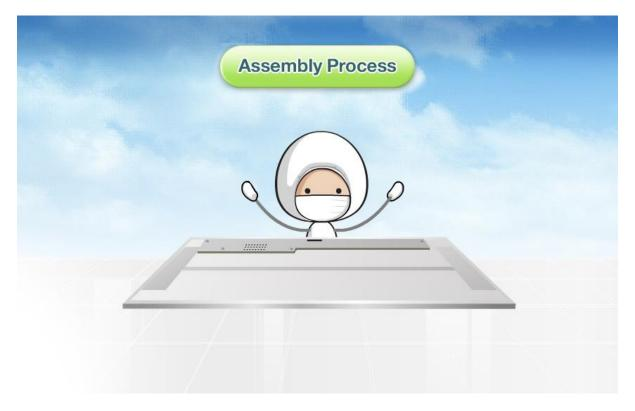
The panel that has gone through the PCB process is called the board assembly. We mount this board assembly on the backlight and fold the PCB back. A top case is placed to fix the panel and the backlight in place and to protect them from external shock. After attaching the film to protect the screen of the panel and assemble a protective case for the PCB, we finally have a TFT-LCD module.
