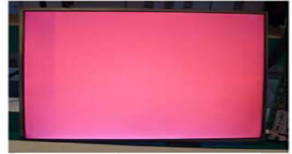
Vertical Block Source TAB IC Defect
