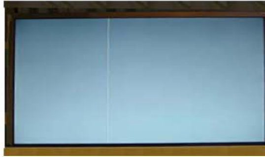
Vertical Line Source TAB IC Defect
