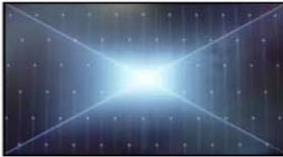
Solder defect, Short/Crack
