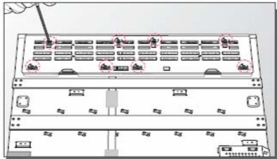
11 Attach the Cover Shield and Assemble the Screw(8EA).
