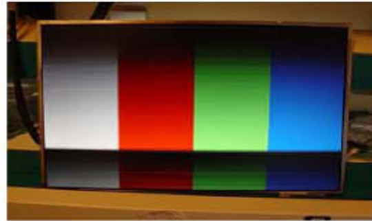
Horizontal Block Gate TAB IC Defect
