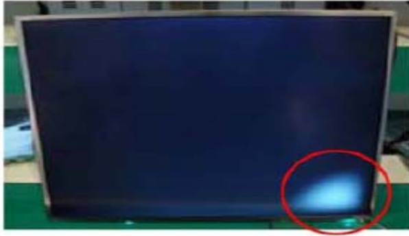
Panel Mura, Light leakage
