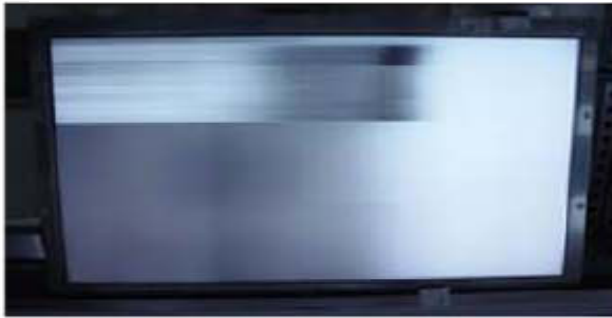
Horizontal Block Gate TAB IC Defect
