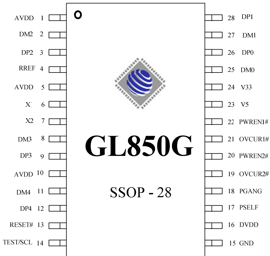
Figure 3.2 – GL850G SSOP 28 Pin Pinout Diagram
