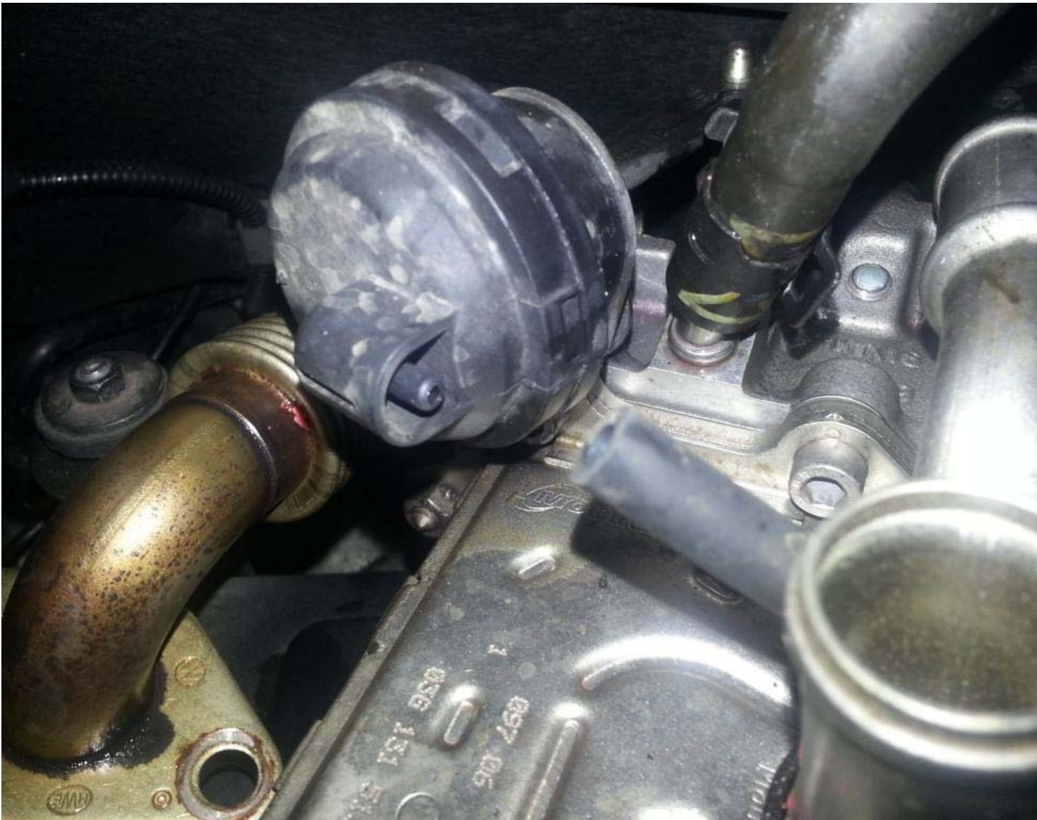
Boost pressure solenoid vacuum hoses.
