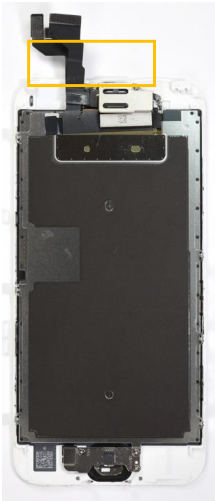
proximity sensor (mnf. unknown) 2.78 mm x 2.38 mm x 1.28 mm
