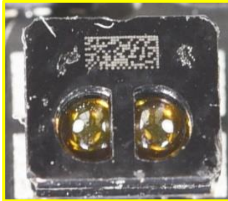
proximity sensor (mnf. unknown) 2.78 mm x 2.38 mm x 1.28 mm
